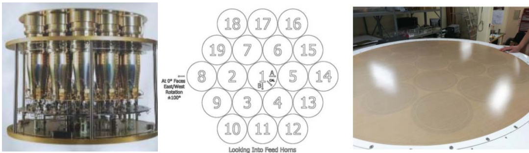
Figure 2.1 The L-band 19 Beam Receiver.
